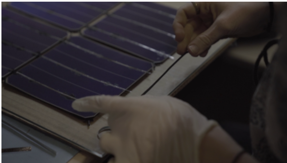
Figure 9. Application of the butyl tape around the edge of the panel
