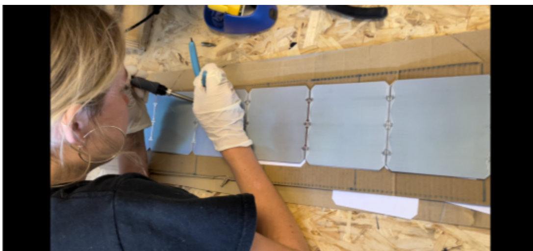
Figure 3. Our social media expert soldering IBC cells.
